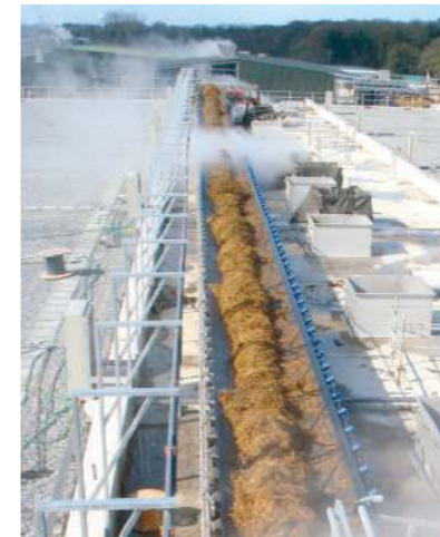
Central conveyor with Discharge wagon. Used to supply a Top filling system.
